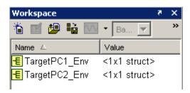
You can save the target PC environment structure to a MAT-file. This enables you to reimport the configuration defined in the structure into a future xPC Target Explorer session.
