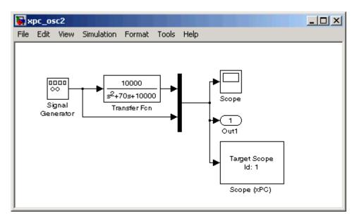
The Simulink block diagram opens for the model xpc\_osc2.mdl.
